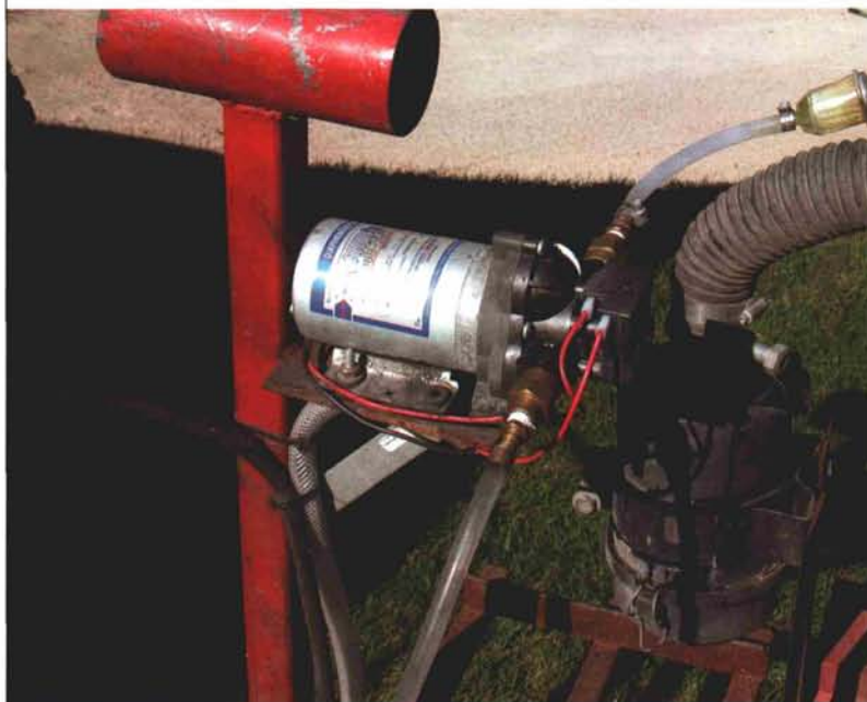
A small 12-volt diaphragm pump supplies water to the misting nozzles. An inexpensive in-line automotive fuel filter removes any debris in the water that could clog the nozzles.
