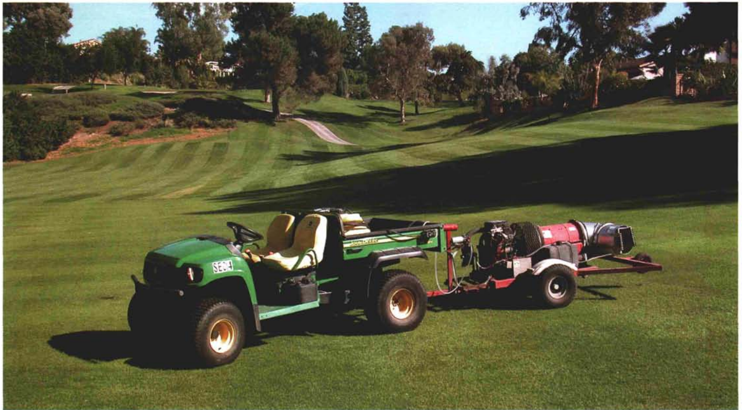
Kevin Hutchins at Mission Viejo Country Club fabricated a syringing system for greens using a utility cart and Buffalo Turbine Blower to help them save time on weekends and minimize interference with golfers.
