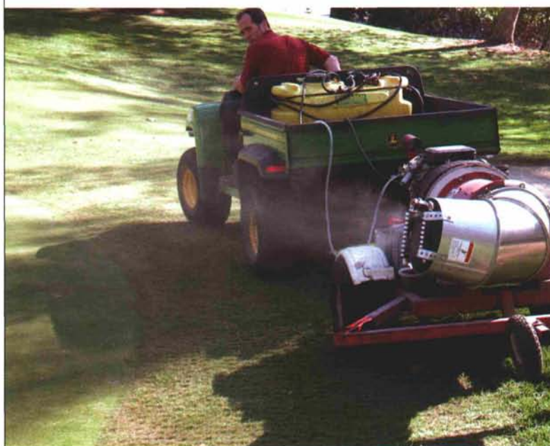
The staff at Mission Viejo Country Club typically uses this setup on Saturday and Sunday afternoons. With two passes around a green, it is possible to reduce surface temperatures by 16°F.
