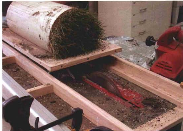
In the fall of 2000, 56 polyvinyl chloride microplots were installed in the plot area adjacent to the lysimeters. Microplots were extracted and partitioned into verdure, thatch, roots, and soil on seven sampling dates to evaluate the fate of labeled nitrogen among turfgrass and soil components.
