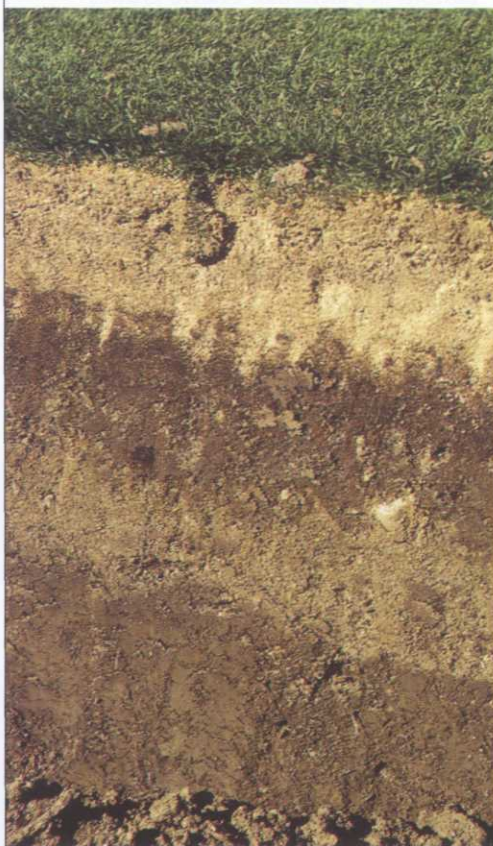
The putting greens had been topdressed for several decades with the same sand used to build the new greens.
