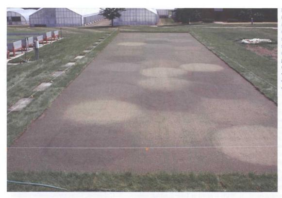
Research at Ohio State investigated quantifying irrigation water savings by using peat or both peat and soil as amendments to highsand-content putting green rootzones. The experimental greens were constructed using wading pools, and the various rootzone mixtures were evident as the plots were grown in.
