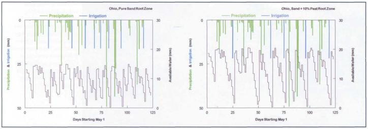
Research analyzed when, given the local climate, an irrigation event was needed to refill the available water capacity and avoid drought stress. The figures show the results from a pure sand rootzone and a sand + 10% peat rootzone at a threshold of 70% available water capacity (AWC). Precipitation and irrigation amounts extend downward from the top, and the present state of available water extends upward from the bottom.
