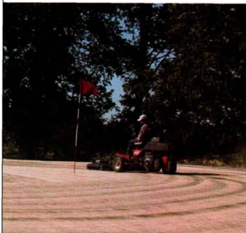
To reduce excessive accumulations of organic matter in putting greens, many superintendents apply a large volume of topdressing material following core aeration.
