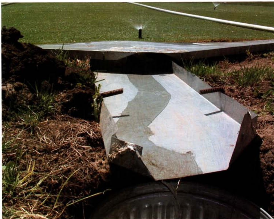
Following pesticide application, irrigation was applied until all plots produced at least 40 liters of runoff.
