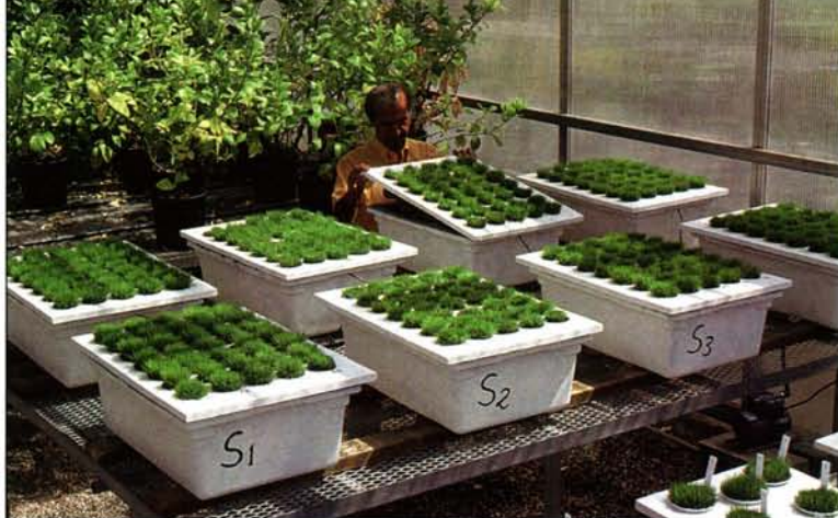
A greenhouse hydroponic system was used to investigate turfgrass salinity tolerance. This system allows for precise control of salinity levels, and both shoot and root responses to salinity can be monitored.
