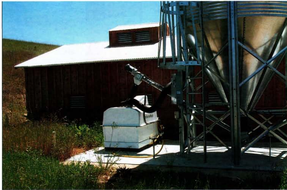
Gypsum injectors are typically used to treat sodic or saline-sodic soil conditions, water sources with high SAR, or very pure water sources.
