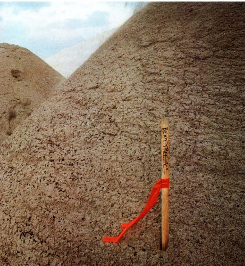
Three 50-ton piles are mixed with varying percentages of organic matter. The piles are "lean," "medium," and "rich." By sampling each pile, the ideal mix can be identified by the laboratory.
