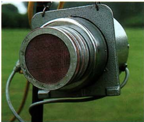
Using an air sampler to collect vapors from evaporated pesticides, researchers evaluate how environmental conditions impact pesticide evaporation loss.
