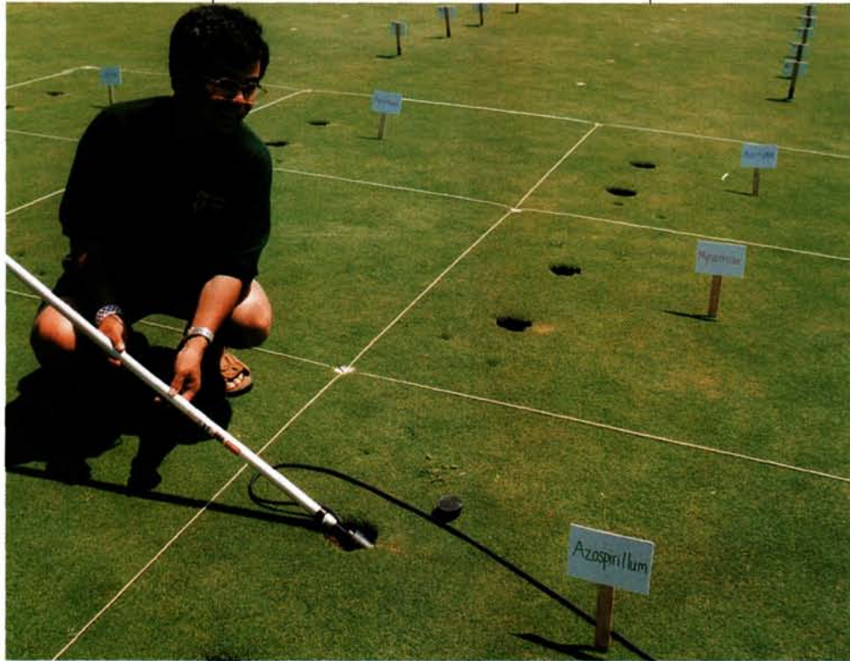
To capture, record, and analyze root images, a video camera is mounted in a tube and inserted into plexiglass tubes buried in field research plots.
