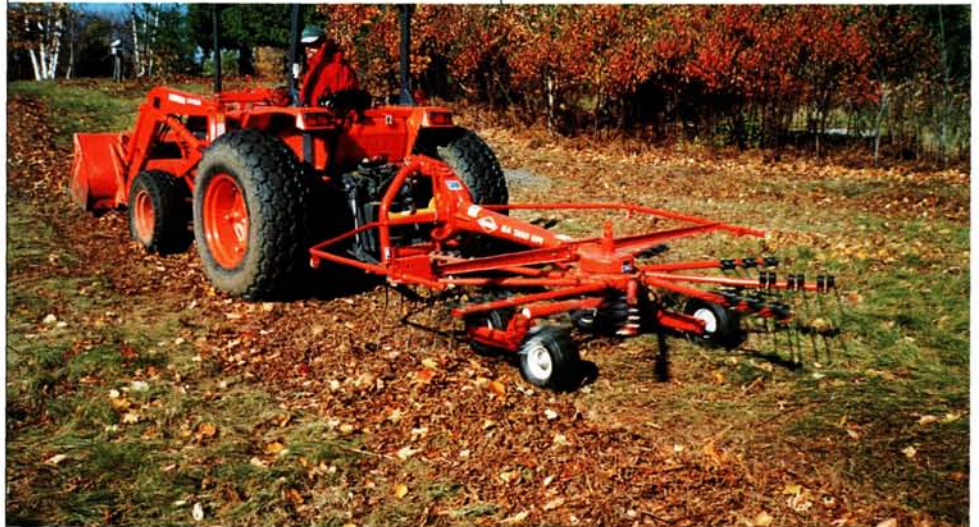
Removing dense clumps of plant debris from mowed sites is a time-consuming operation unless specialized equipment is used. A Kuhn rake will windrow plant debris and the tines will further thin out dense stands of native grasses.
