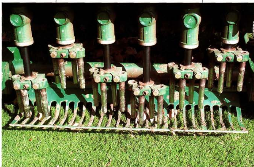
The quadra-tine holder was modified to accept a larger ½" hollow aerification tine. It now has the capability to impact a larger amount of surface area.
