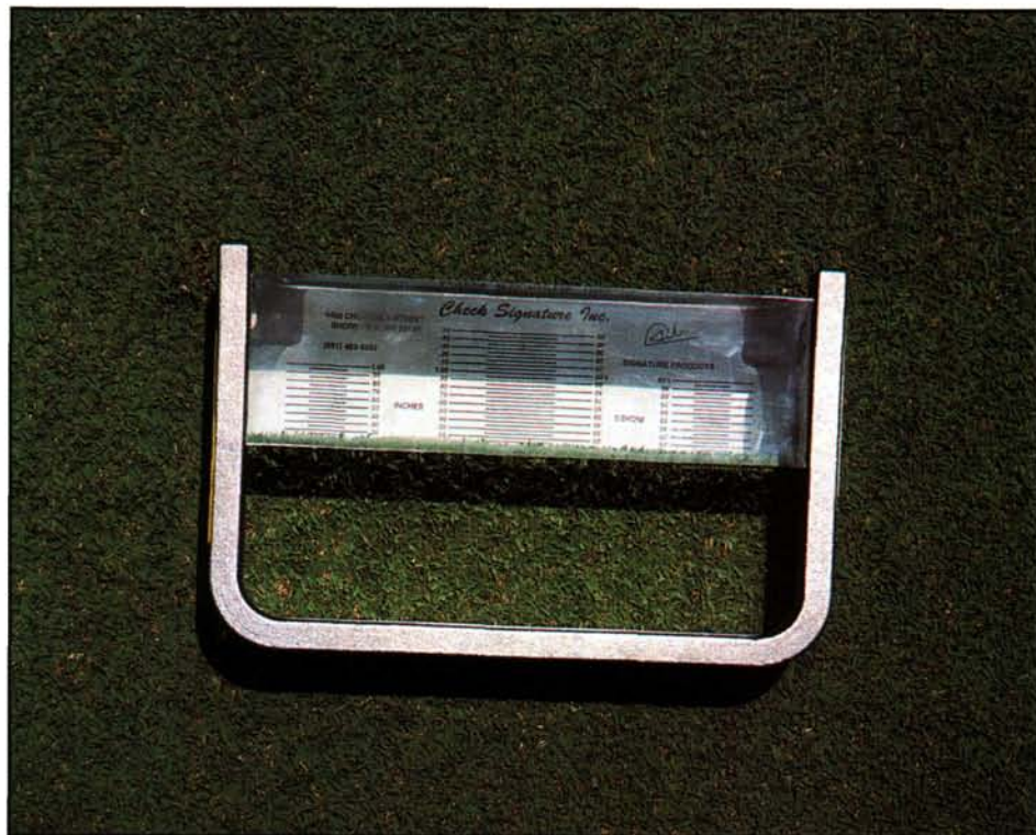
What is the effective height of cut? Prism gauges are a useful tool for determining the actual mowing height.
