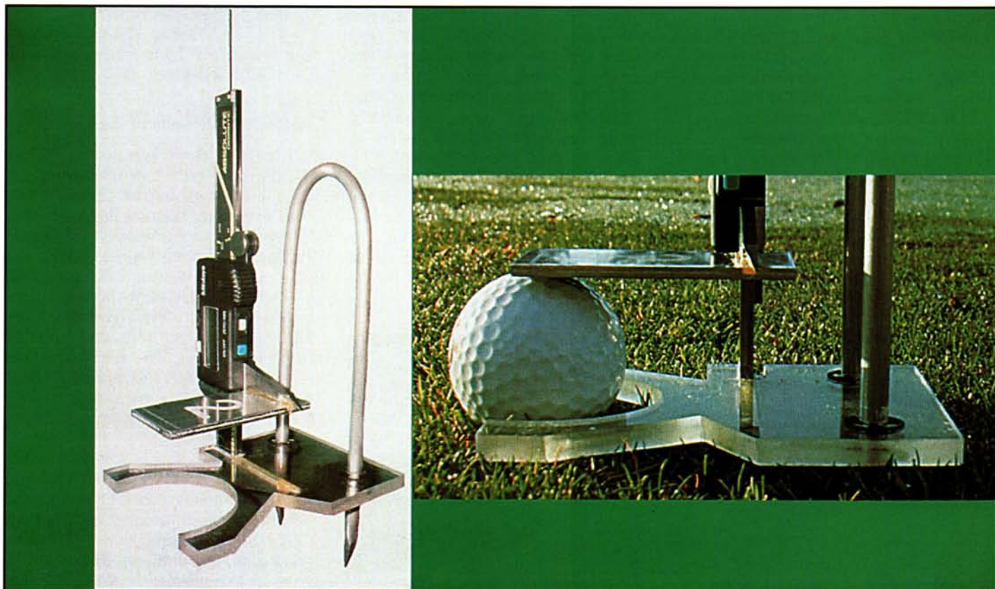
Lie-N-Eye is a device developed by University of Illinois researchers to measure the ability of a turfgrass species to support a golf ball under a typical fairway setting.
