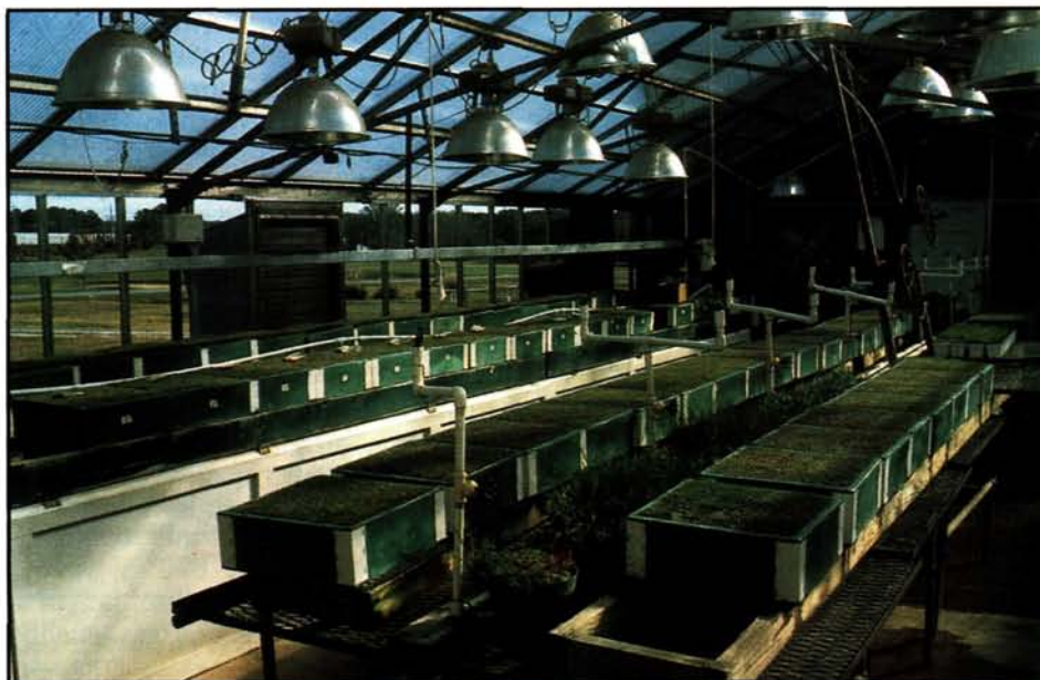
Simulated golf greens were constructed in the University of Georgia greenhouse and used for studying nitrogen and phosphorus leaching through the soil
