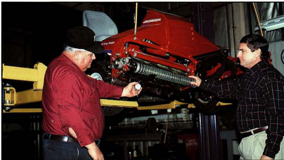
A properly equipped maintenance facility includes a hydraulic lift in the mechanic's work area. This investment allows equipment repair and servicing to be performed rapidly and efficiently.
