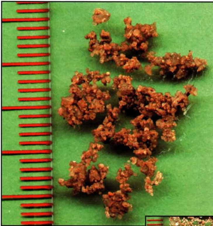
The amount of silt and soil in bunker sand impacts drainage capabilities. A high-resolution scan of a bunker sand that drains properly (right) compared to a slow draining bunker sand will probably show the presence of silt and soil (above).
