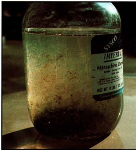
Excess suspended solids can plug water-conducting pores at the soil surface. Low-quality effluent irrigation sources are notorious for containing high loads of suspended organic solids.
