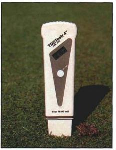
New, low-cost meters are available to help superintendents better manage their courses. The TDSTestr 4<sup>™</sup> meter measures salt accumulation in the root zone from saline irrigation supplies and lets superintendents know when overirrigation is required to prevent turf damage.
