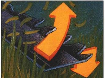
The genius of the Gator Mulcher™ blades is the four louvers on the opposite side of the cutting edge. These louvers redirect a high percentage of the air flow towards the center of a standard deck so that large clippings and other debris are re-cut over and over.
