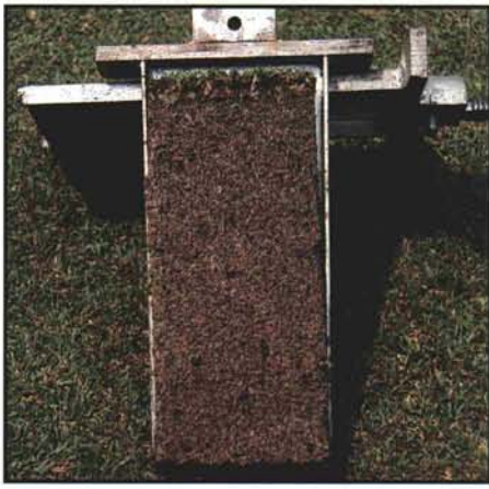
A good root zone mix is the baseline for quality greens, but it is critical that a proper layer of thatch develop to provide resiliency and good putting qualities before opening new greens for play.
