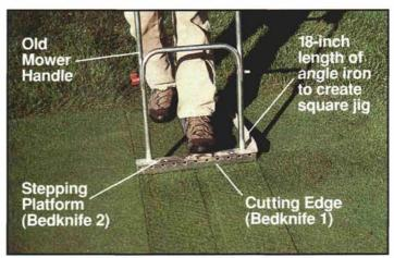
Two bedknives, an 18-inch length of one-inch angle iron, and an old lawn-mower handle were used to create this tool which cuts perfectly square pieces of sod. The 18-inch square pieces are easy to handle and fit well together.
