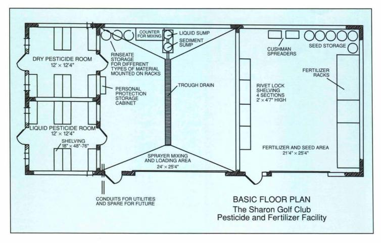
Each room has two sets of doors. One door opens directly into the mix-load area. The second door opens to the outside, which is a fire code requirement.
