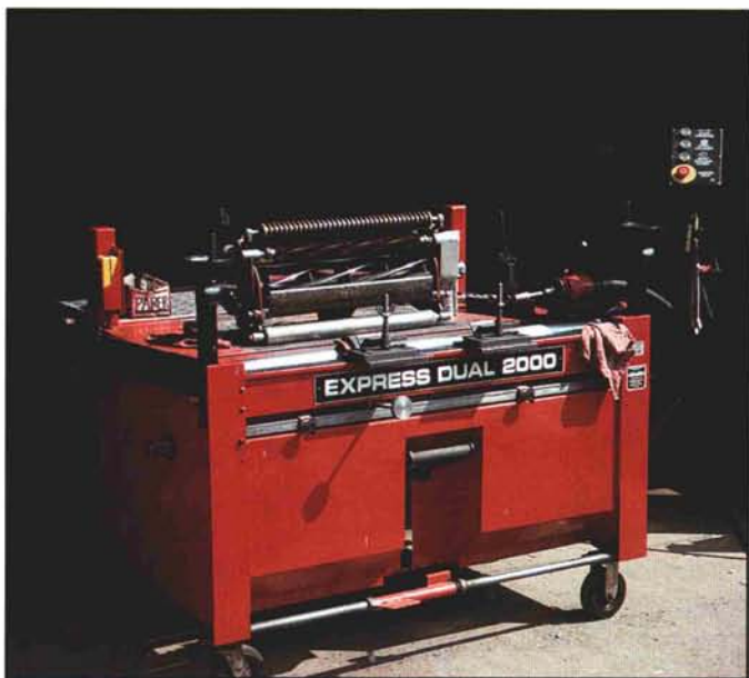
Newer grinding equipment provides the flexibility to sharpen mowers during the season in a very short period of time.
