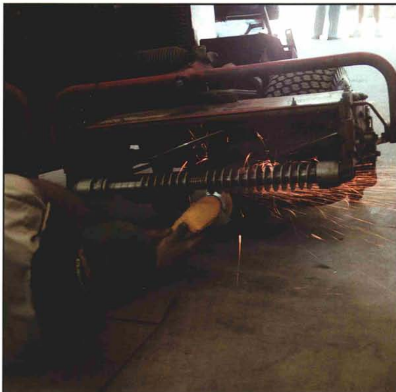
During the golf season, a body grinder can be used to maintain a sharp face on the bedknife. In the hands of an experienced mechanic, five minutes is all that's needed to make the mower ready to go!
