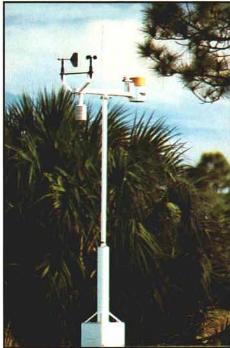
Weather stations located on the golf course provide valuable information that is used in irrigation programs. See page 18.
