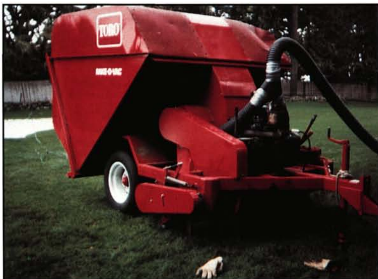
The 4-inch-diameter drain lines were inserted into the access ports on each side of the blower housing. After operating the turf vacuum for six hours, the staff had sufficiently dried the soil profile and alleviated the black layer.
