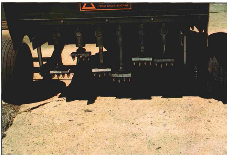
(Above) Developments in aeration accessories, such as solid-tine aeration with the Job-Saver attachment, give the superintendent flexibility to accomplish various tasks. (Left) Shallow aeration can be accomplished using hollow tines on the Core Master.
