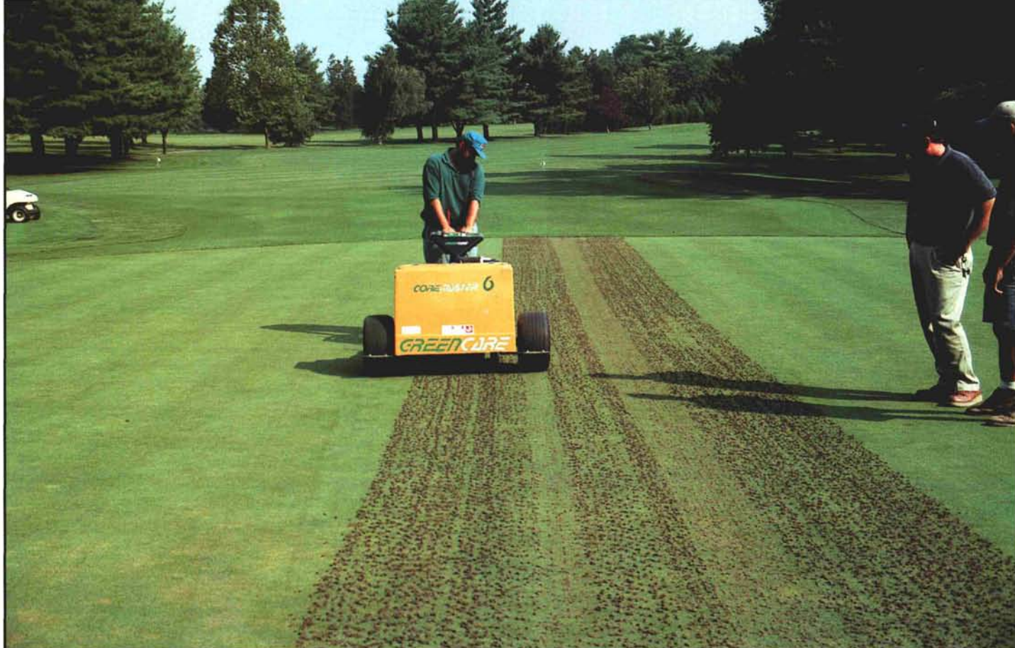
(Above) Developments in aeration accessories, such as solid-tine aeration with the Job-Saver attachment, give the superintendent flexibility to accomplish various tasks. (Left) Shallow aeration can be accomplished using hollow tines on the Core Master.
