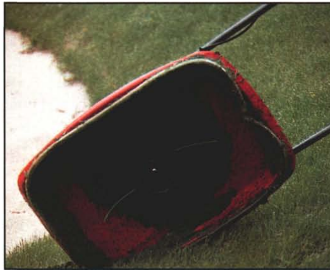
A Flymo is modified with \frac{3}{8} -inch vinyl tubing to elevate the machine for a greater height of cut.
