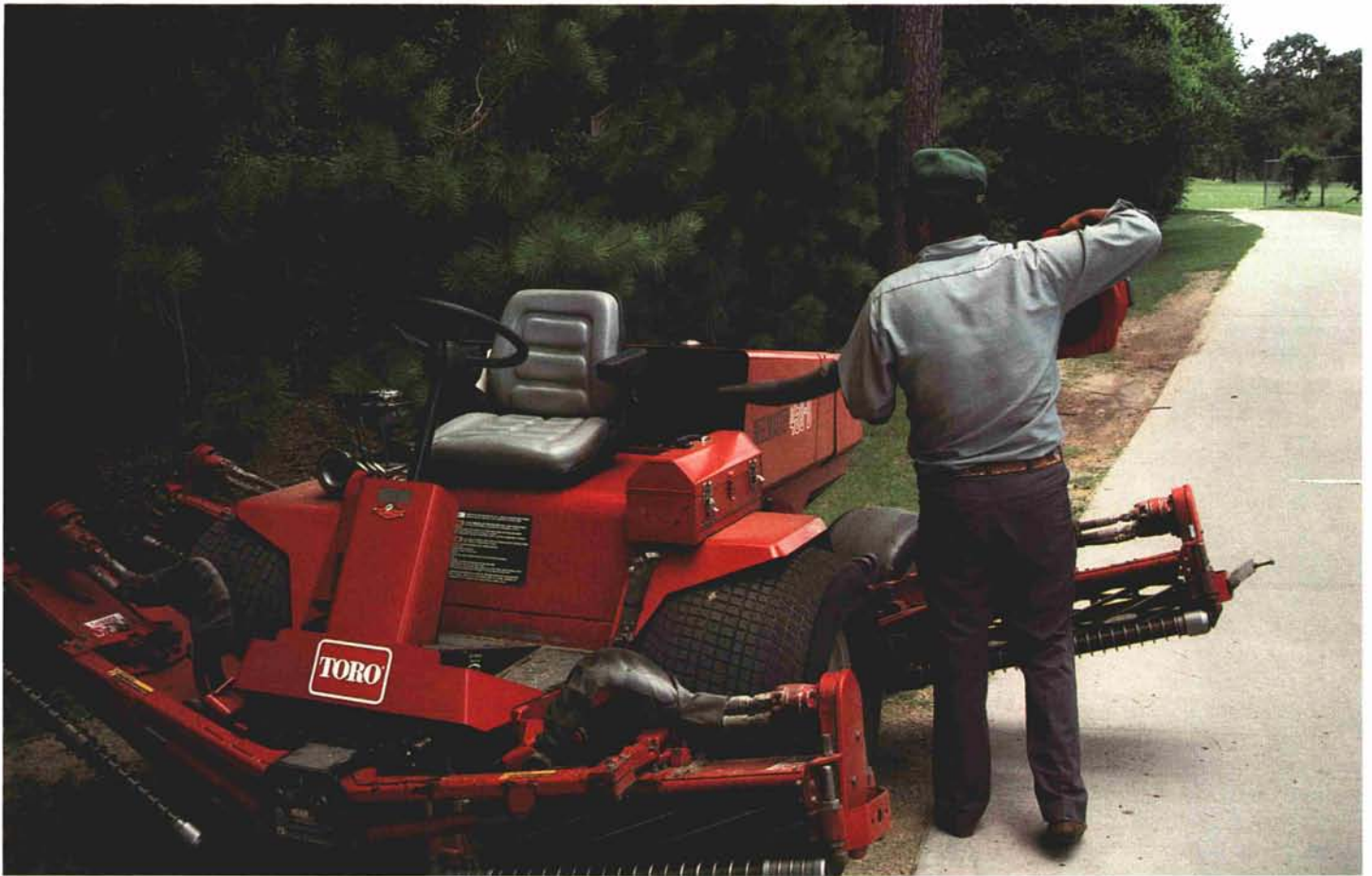
Simply blowing the equipment clean eliminates most of the clippings from the unit.
