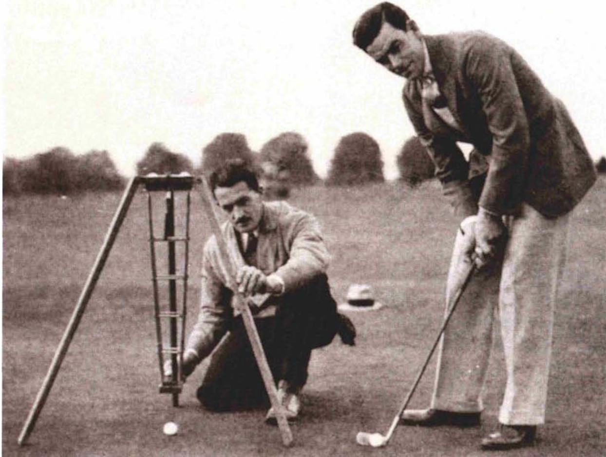
Dr. Fred Grau (left) and Johnny Farrell (1928 U.S. Open winner) used a mechanical putter in 1933 to test the putting quality of USGA grasses located at the Arlington turf garden, Arlington, Virginia. The mechanical putter eliminated the human factors when measuring drift and ball speed.
