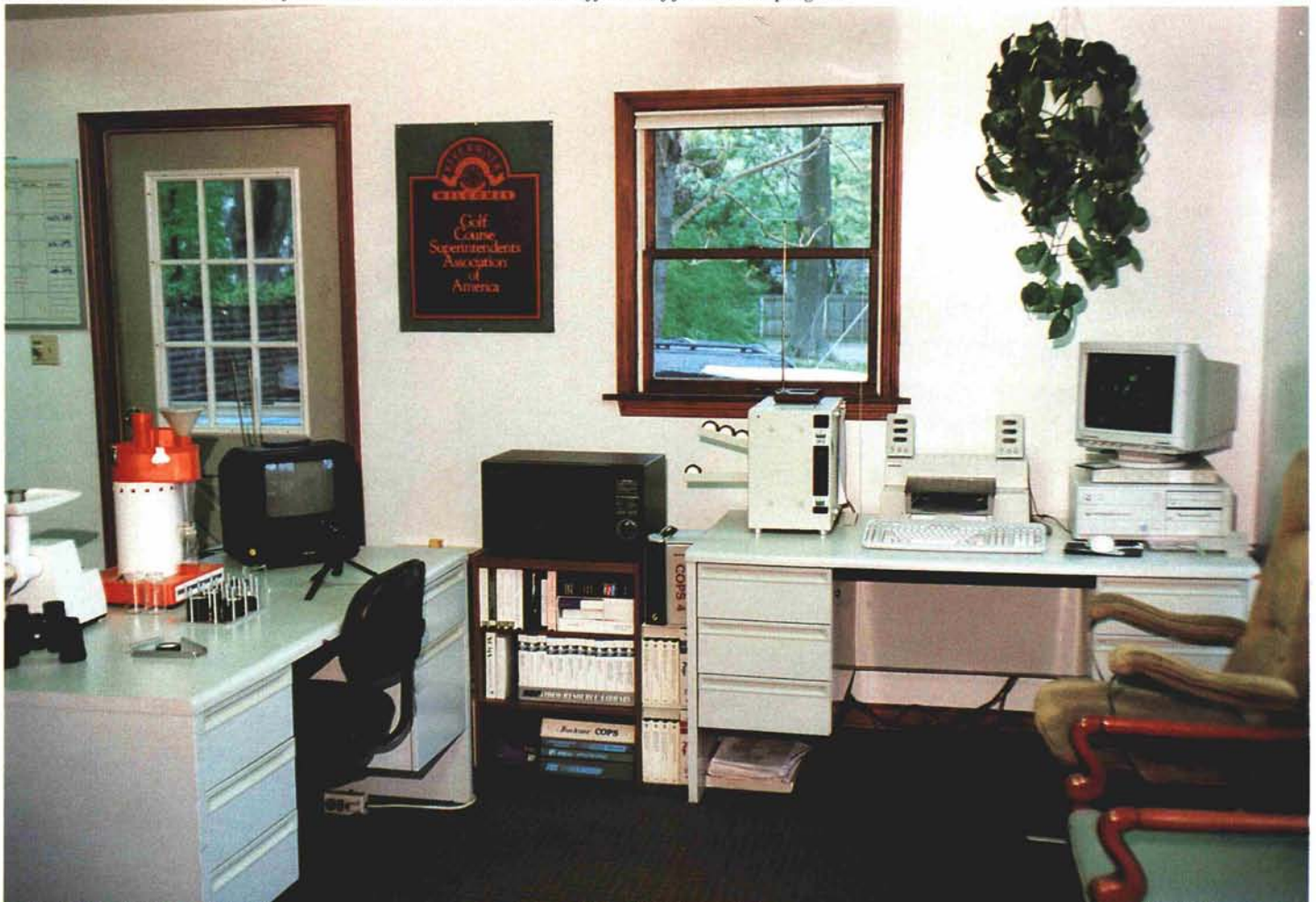
The Old Westbury Golf and Country Club uses in-house near-infrared spectral (NIRS) analysis to measure essential nutrients in leaf tissue. The results are used to modify the turf fertilization program.
