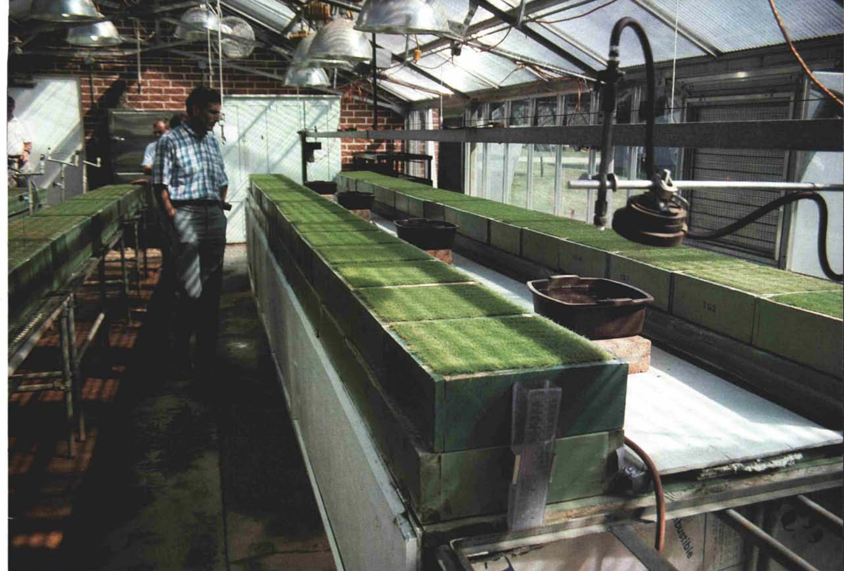
These greenhouse lysimeters were used to obtain information about pesticide leaching through turfgrass profiles. University of Georgia.
