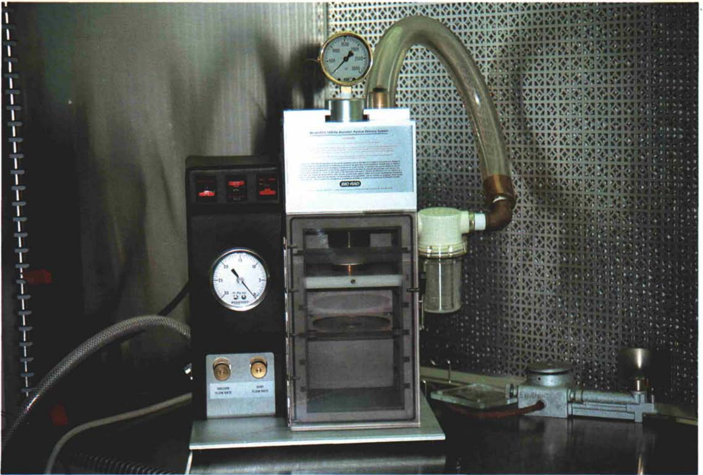
Highly specialized equipment is used to shoot foreign DNA into bentgrass plant cells.
