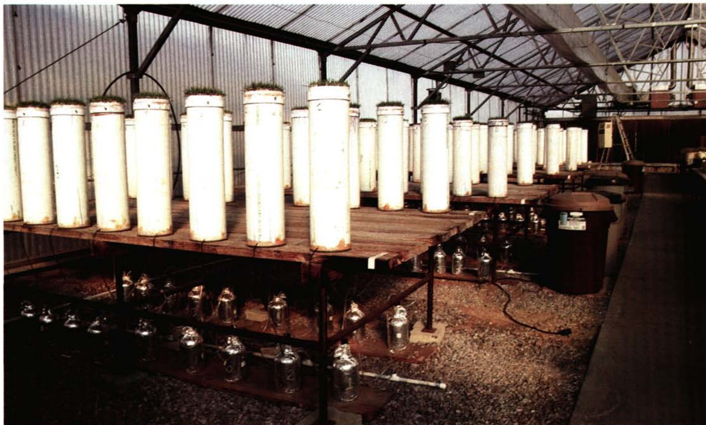
Column lysimeters planted to tall fescue or bermudagrass used to collect leachate in the greenhouse portion of the study.
