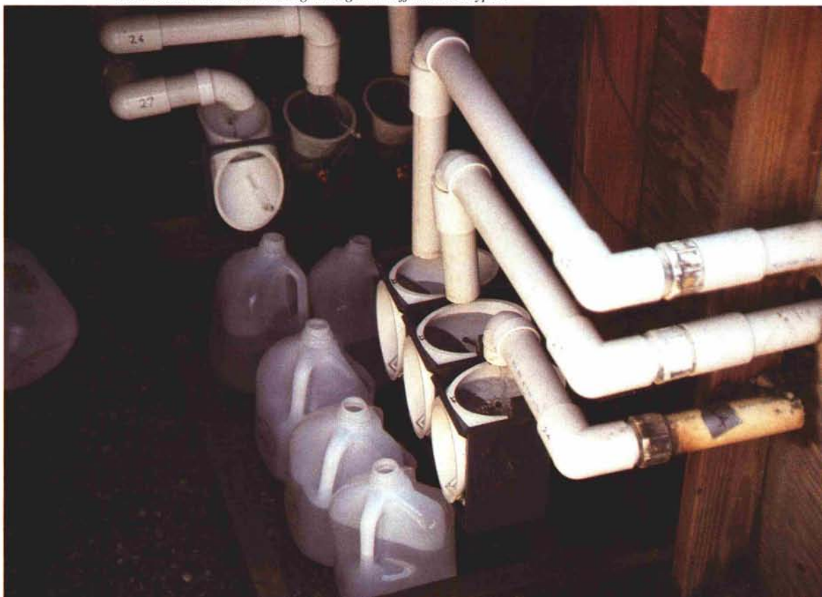
Each lysimeter has an individual collection port to sample and monitor the water moving through the different soil types.
