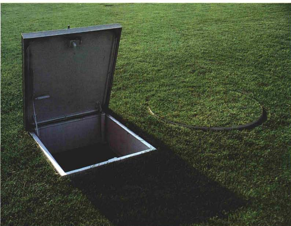
Before (top) and after (above). Stainless steel lysimeters were installed without disturbing the soil profile in the cylinder. An adjacent access port enabled researchers to collect samples.
