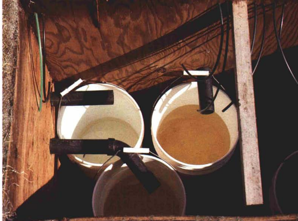
The leaching collection system from the lysimeters provides turfgrass scientists the ability to closely monitor the inputs and outputs from the system. The project at Washington State University studied amended versus non-amended sands with varying N fertilization rates.
