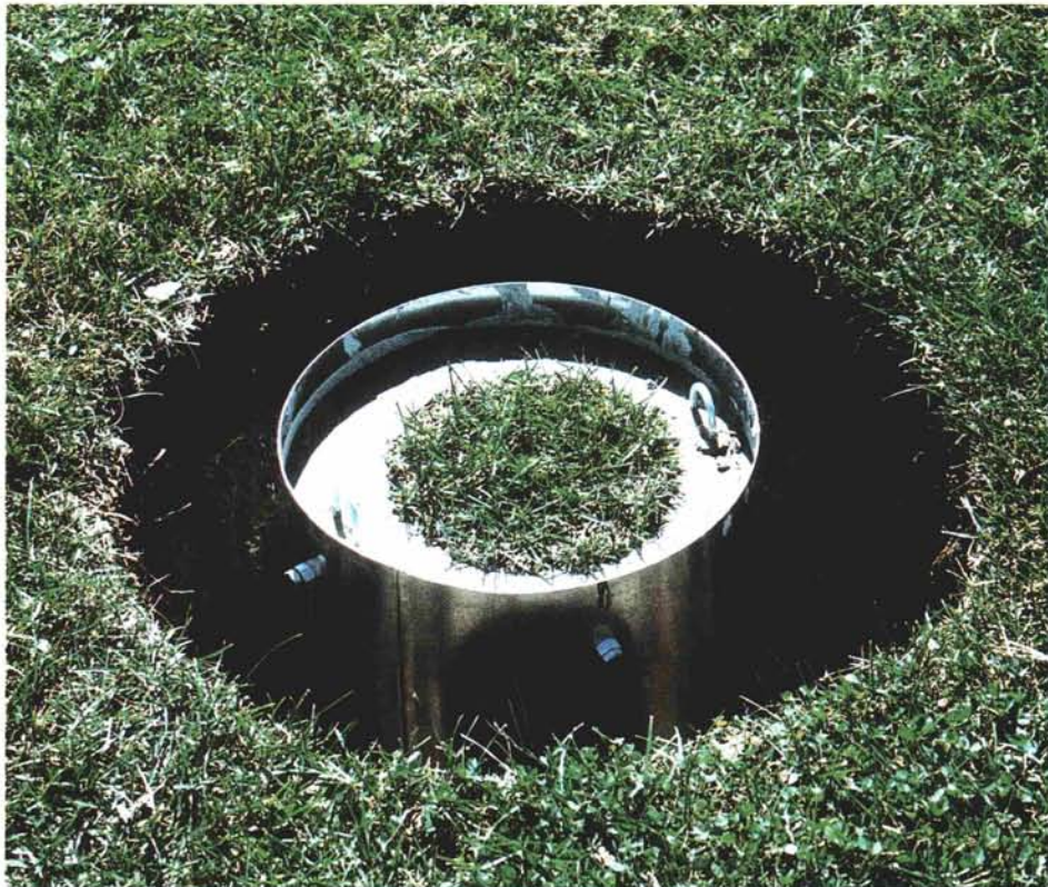
Encasement of the turf/soil column ensures an intact undisturbed profile for pesticide sampling.
