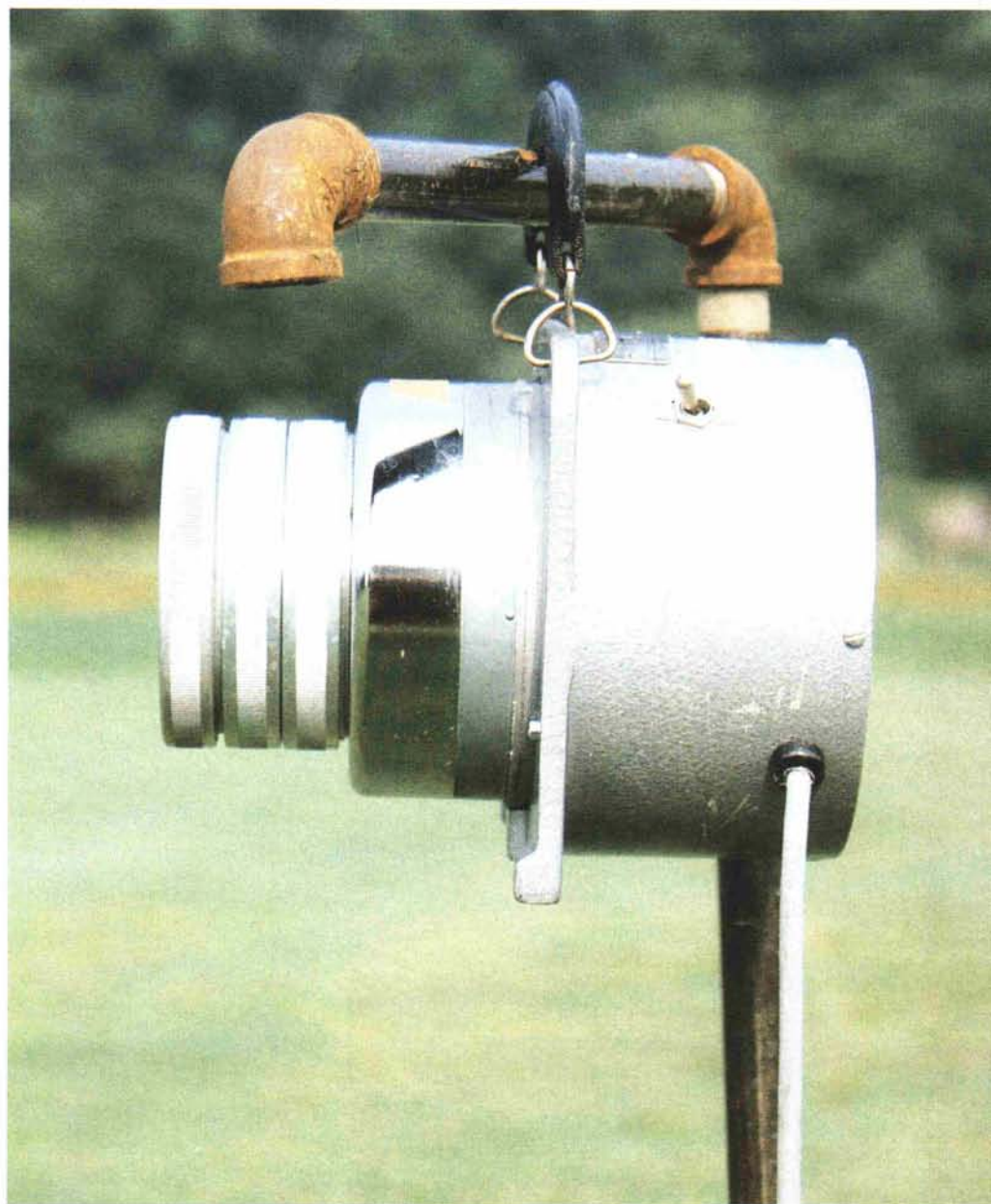
Figure 1. A high-volume air sampler was used to collect volatile loss of pesticides.
