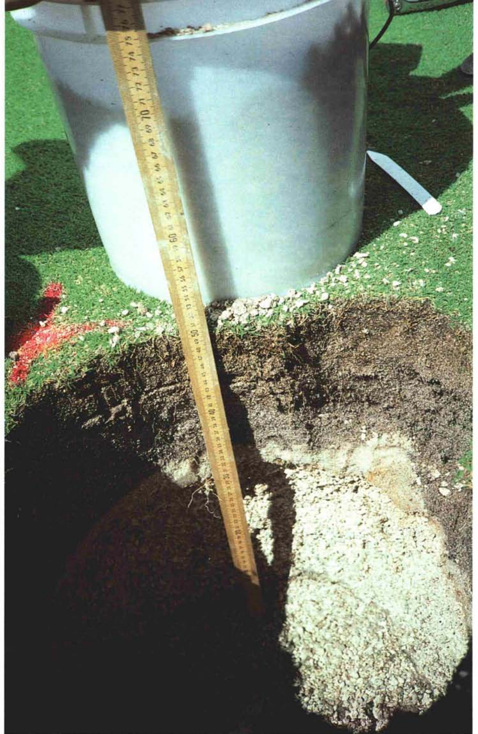
The gravel, very coarse sand, and root zone mix depths were measured in the green so that the same depths could be reproduced in the lysimeters.
