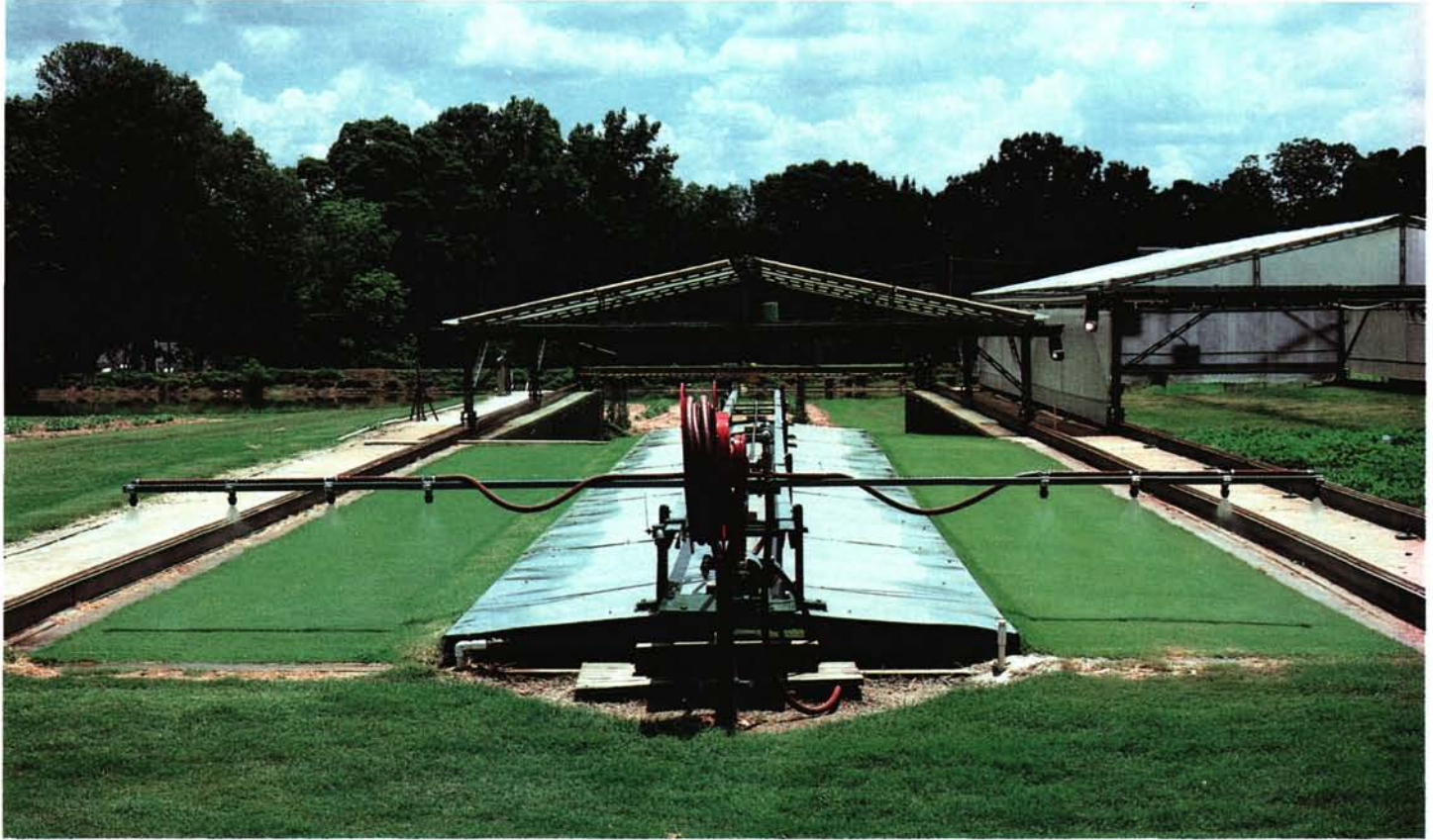
Field lysimeters, maintained as a green, used both bentgrass and bermudagrass. An automatic rain shelter protected the lysimeters from natural rainfall events.
