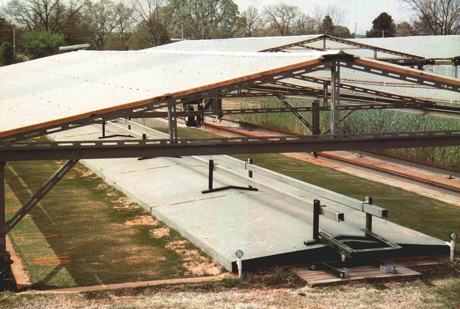
Dr. Al Smith, University of Georgia, is evaluating the fate of pesticides applied to bermudagrass and bentgrass putting greens. The lysimeter facility contains a series of buckets (not shown) buried underneath the surface of the green that collect water moving through the soil. Water samples analyzed in the laboratory indicate that the amount of properly applied pesticides passing through putting greens is negligible.
