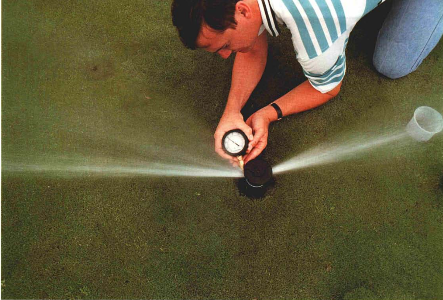
One clear sign of an irrigation system with undersized main lines and laterals is the loss of operating pressure at sprinkler heads located furthest from the pump station.
