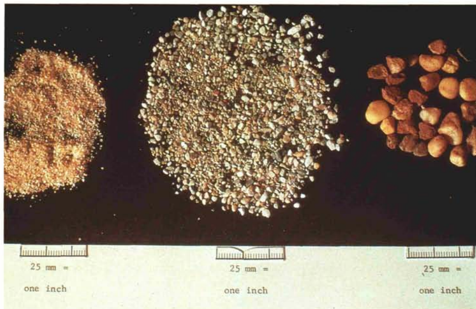
An example of topmix construction materials: topmix sand, intermediate layer sand, and pea gravel. USGA specifications for green construction are the most widely accepted in the turfgrass industry.
