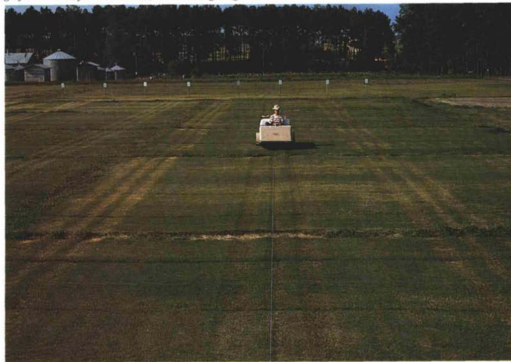
Experimental bermudagrasses were tested for wear tolerance by using different golf cart tires, fertilizer rates, and cutting heights.
