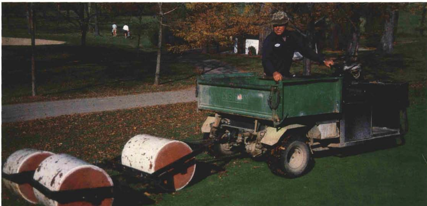
These gang-rollers, tended by assistant superintendent Bert Bertram, contribute to surface smoothness and increase putting speed from 6 to 12 inches.
