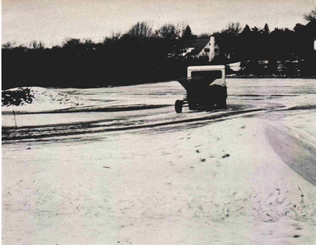
Applying topsoil to greens and surrounding area with a broadcast type fertilizer spreader to prevent winter injury.
