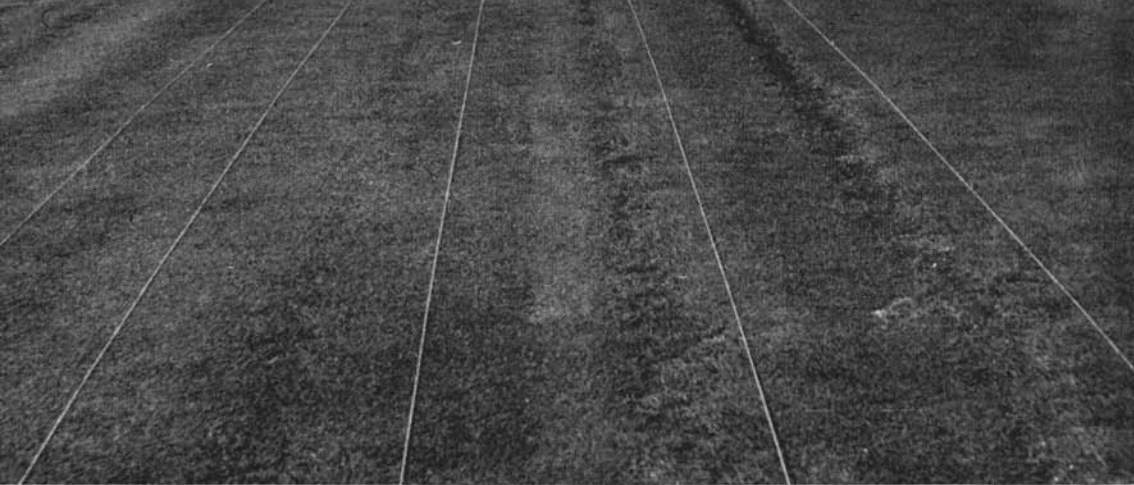
Damage to Seaside bentgrass after 630 traverses during 6 weeks in 1958 by: left—ripple sole shoes; center—rubber lug sole shoes; right—conventional spiked shoes. Ripple sole shoes produced least damage, conventional spiked shoes greatest damage.
