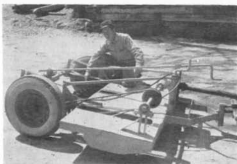
Side view of dallisgrass cutter showing tractor hitch and power take-off arrangement.
